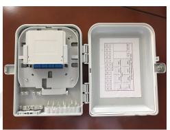
8/16-Core Optical Termination Box is designed to connect feeder/distribution cable to subscriber's drop cable using PLC splitter in FTTx networks. TX-FTTH-618has 2 input output ports on the bottom and it is easy to install on the wall or pole. The rear tray is for splicing a fiber of feeder cable with PLC splitter and the front tray is for connecting subscriber's drop cable through adaptor plate on the tray.
